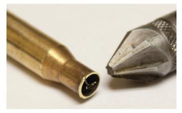
2. The next step will be to adjust the 6.5-06 sizing die to partially size part of the length of the case neck. This may require some fine adjustment. You will want to size only a small portion of the neck and then try chambering in your firearm to
