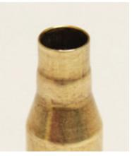
3. Now we are ready to fireform. Pick an appropriate burn rate of powder for the cartridge. Starting just slightly under the midpoint of the powder charge range for the bullet weight you will be using. Load 2 or 3 and fire them in the rifle. If the cases look like the shoulder is formed, and the neck looks filled out, then the charge is sufficient. If not, then increase the powder charge about one-half grain until the case is formed.
