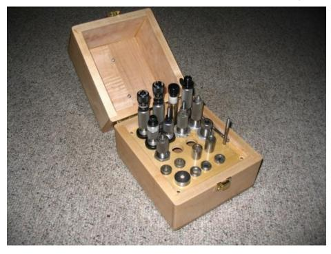
And lastly, how about all of those cast bullet sizing dies and nose punches? The 3-box photos shows a J&J Products ammo box converted to store these items along with cast bullet lube.
